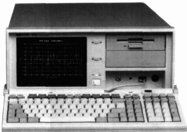
HP R/332 Rackmount Controller
