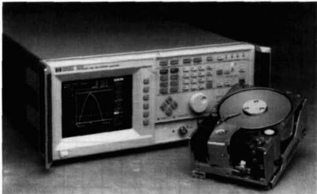
The HP 5372A displays window margin information directly for disk and tape drive testing.
